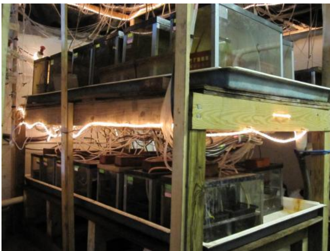
In the Room of DOOM (Dissolved Oxygen Oyster Mortality), oyster tanks mimic the day-night oxygen swings that oysters experience in shallow Bay waters. Credit: SERC
